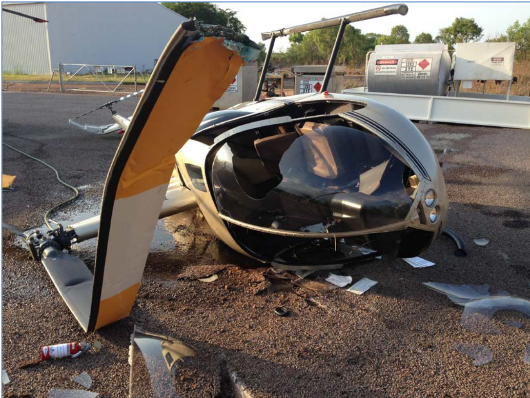
Figure 2: VH-ZWA on right side showing damage to main rotor and cabin
